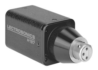
The H187 plug-on transmitter adapts microphones with XLR connectors to wireless operation. The spring-loaded, rotating input coupler is easy to operate, yet provides a firm, noise-free fit with a wide variety of different microphones. The transmitter housing and the body of the attached microphone form an efficient dipole antenna configuration, with an insulator between the input coupler and the lower section of the transmitter housing separating the two halves of the antenna.
