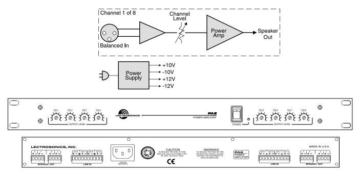
The input to the PA8 is fully balanced and RF filtered. The level control feeds a monolythic power amplifier. Each power amplifier is internally power limited to protect itself from short circuits, excessively low load impedances, or highly reactive loads. Thermal limiting is also integrated into the power amplifier, with an intelligent shutdown mode that minimizes thermal shock to the device under extreme operation.
