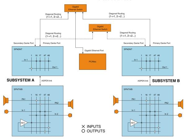
Dante devices configure themselves automatically as soon as they are connected into the network, with a single unit being chosen as Master to generate the system clock and the others configured as Slaves.
