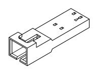
Pin 1- Anode Pin 2- Cathode
