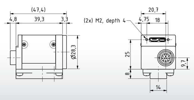
Dimensions: mm Tolerances: DIN ISO 2768m
