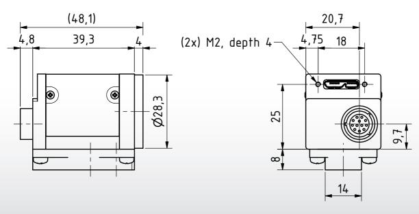
Dimensions: mm Tolerances: DIN ISO 2768m
