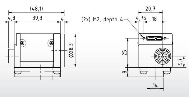
Dimensions: mm Tolerances: DIN ISO 2768m
