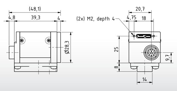
Dimensions: mm Tolerances: DIN ISO 2768m
