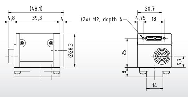
Dimensions: mm Tolerances: DIN ISO 2768m
