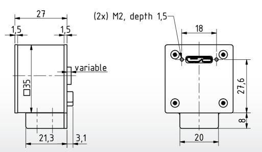
Dimensions: mm Tolerances: DIN ISO 2768m
