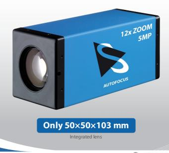
The Imaging Source DFK Z12G445 color camera has a GigE interface and is the perfect solution for many industrial automation, quality assurance, security, surveillance and medical applications. The color camera ships with the very sensitive 1/3 inch Sony CCD ICX445AQA sensor. With up to 30 images per second, the DFK Z12G445 is a low cost, yet highly versatile imaging solution. The camera integrates an autofocus lens (Automatic/manual)
