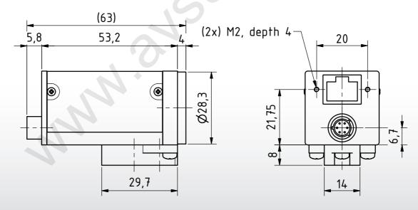
Dimensions: mm Tolerances: DIN ISO 2768m
