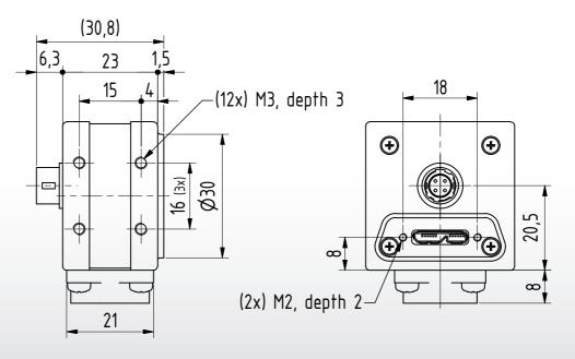
Dimensions: mm Tolerances: DIN ISO 2768m
