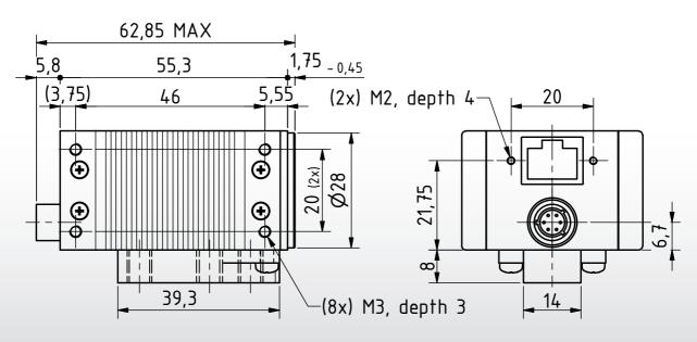
Dimensions: mm Tolerances: DIN ISO 2768m
