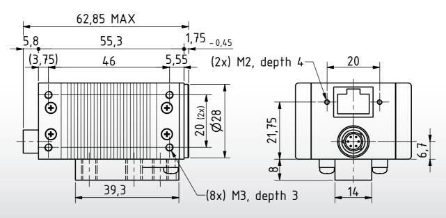
Dimensions: mm Tolerances: DIN ISO 2768m
