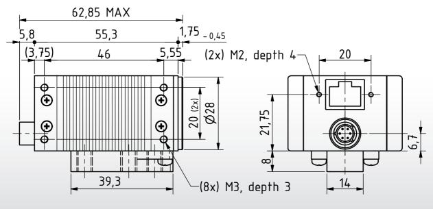
Dimensions: mm Tolerances: DIN ISO 2768m
