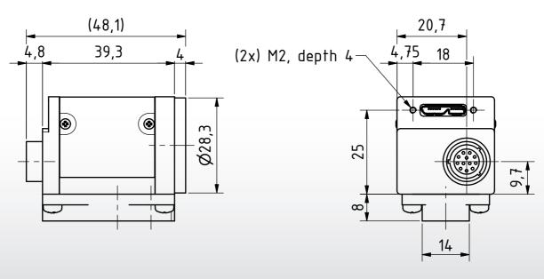
Dimensions: mm Tolerances: DIN ISO 2768m
