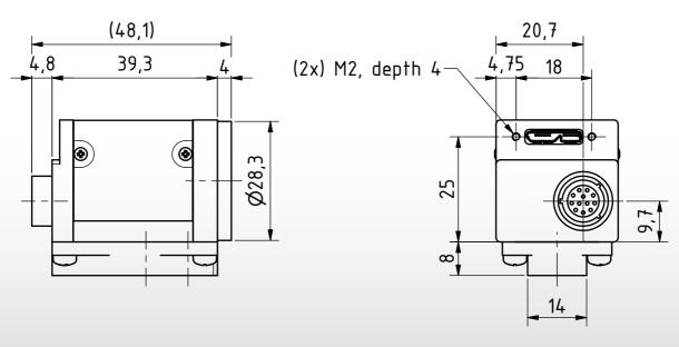
Dimensions: mm Tolerances: DIN ISO 2768m
