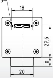
Dimensions: mm Tolerances: DIN ISO 2768m
