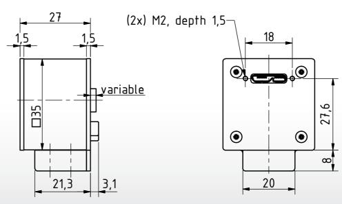
Dimensions: mm Tolerances: DIN ISO 2768m
