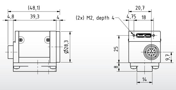
Dimensions: mm Tolerances: DIN ISO 2768m
