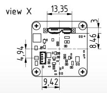
Dimensions: mm Tolerances: DIN ISO 2768m
