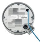
Only a single Ethernet cable is needed to connect the IK-WR14A to the network and electrical power
