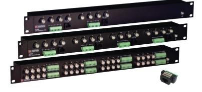
The Vigitron Vi1008, Vi1016 and Vi1032 are 8, 16 and 32-channel passive transceiver hubs that transmit or receive video signals over unshielded twisted pair (UTP) wires, point-to-point, for distances up to 1,000 ft. (305 m)\*. They are used with any Vigitron transceivers to support "up-the-coax" PTZ signals. These hubs use category 2-7 twisted pair wires, and are easy to install, cost effective and do not require power.
