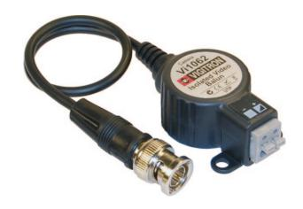
The Vigitron Vi1062 is a passive transceiver that includes a built-in video isolation transformer and transports video signals over unshielded twisted pair wires, point-to-point, for distances up to 750 feet (228 m). Distances up to 3,500 feet (1,066 m) can be achieved when it is used with Vigitron active UTP receivers. It uses Category 2-7 twisted pair wires, is easy to install, cost effective, and does not require power.
