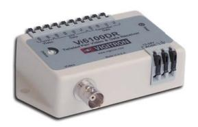
The Vigitron Vi6100DR is an advanced active device that receives color or B&W video and data over separate point-to-point unshielded twisted pair wires at distances up to 6000 feet (1830 m). The Vi6100DR uses Category 2-7 twisted pair wires, is easy to install and cost effective. It is designed to be paired with Vigitron Vi6100DT active video and data transmitter.
